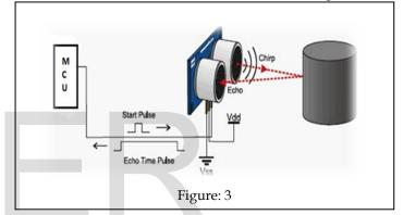
precise, non-contact distance measurements from about 2 cm (0.8 inches) to 3 meters (3.3 yards). It is very easy to connect to microcontrollers requiring only one I/O pin [4].
